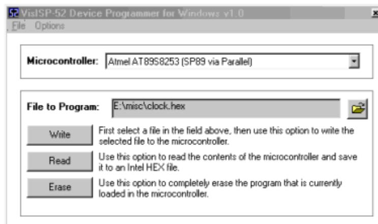
Before proceeding, make sure you've selected the right microcontroller in the "Microcontroller" drop-down window. At this time, VisISP-52 only supports the Atmel AT89S8252 and AT89S8253.
