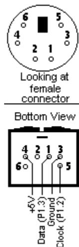
This program requires a PS/2 keyboard to be connected to the SBC. The keyboard requires a +5V power supply, ground, and the program assumes that the keyboard data line is attached to P1.3 and the clock line is attached to P1.2.
