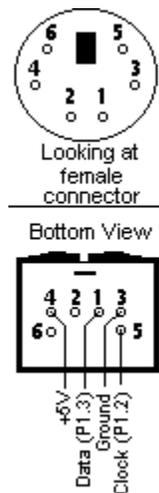
This program requires a PS/2 keyboard or mouse to be connected to the SBC. The keyboard requires a +5V power supply, ground, and the program assumes that the keyboard data line is attached to P1.3 and the clock line is attached to P1.2.
